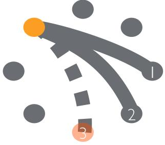
Even though node 3 fails, there are two copies still stored and any node will accept a write for the failed node.
