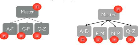
4 SPOF vs. 5 SPOF ...you end up less fault-tolerant!
