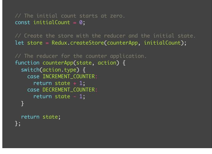
So here we see the creation of the store with an initial value of zero. The "counterApp" is what Redux called a Reducer, a Reducer takes the state and an action payload and performs the action on the state.
