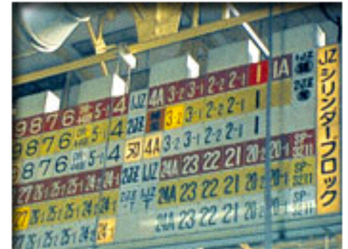
An andon problem display board that communicates abnormalities
